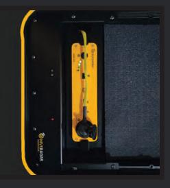
2. Power up. Connect the 12 volt plug into the receptacle on the battery. Press and hold the button unti the indicator lights come on\*. Check the small indicator lights\* on the PowerPack below the battery to ensure that the PoE injector has power.
