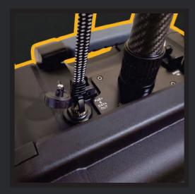
**9.** Connect the other end of your ethernet cable to the ethernet port labeled "PoE+ & data out"
