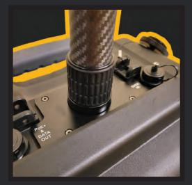
7. Connect the remaining poles. Unscrew the cap at the top of the case and screw in the lower pole assembly.
